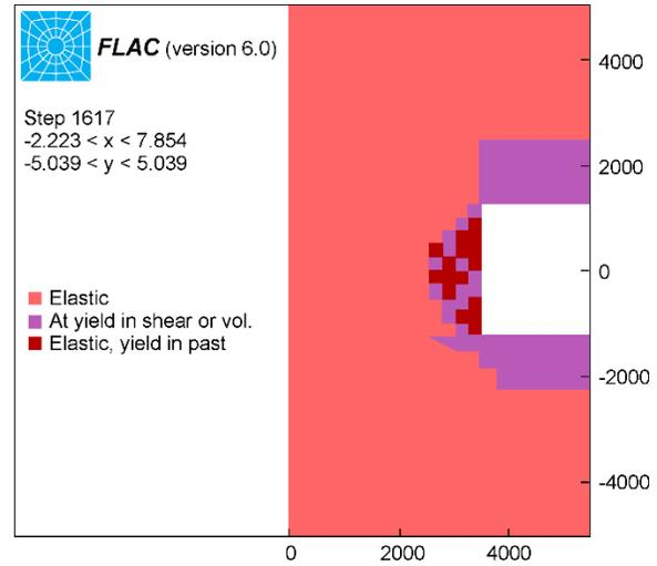
Figure 7: Yielding around a pillar in the case of a poor quality rock mass.
