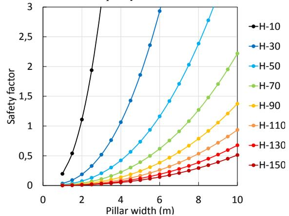
Figure 6: Safety factor as a function of pillar width for various mining depths.
