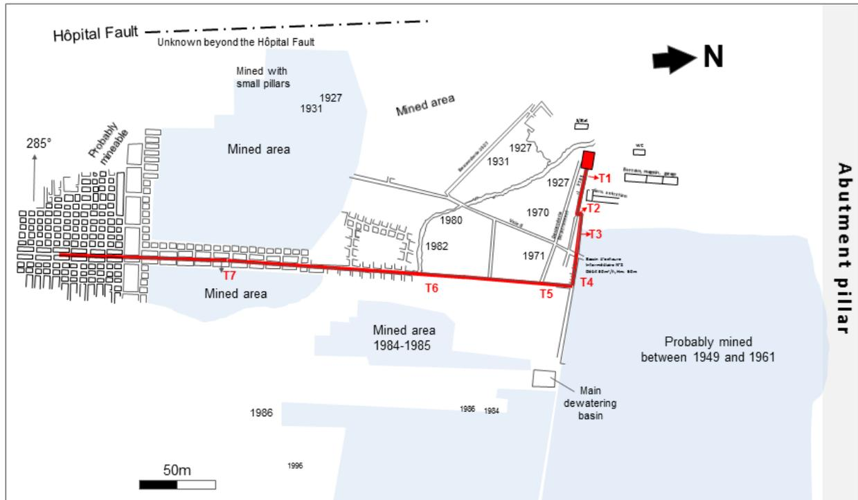
Figure 3: Mining map at Makala. In red, the main access from surface to the face.
