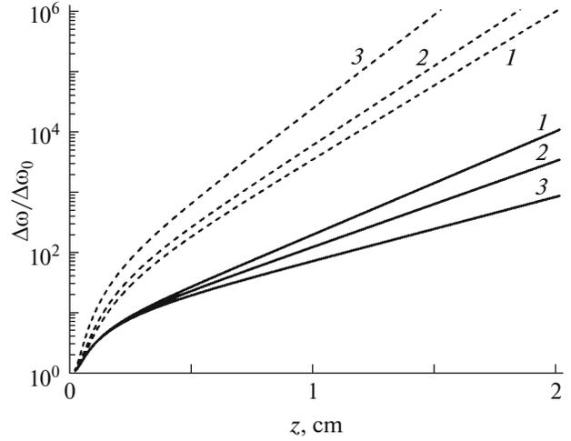
**Fig. 2.** Normalized spectral width as a function of waveguide length at  $b = -3 \times 10^{-4}$  and  $D_z = (0.5, 0.9, 1.3) \times 10^{-21}$  s<sup>2</sup>/m (solid lines 1–3, respectively); at  $D_z = 1 \times 10^{-21}$  s<sup>2</sup>/m and  $b = (-2, -2.3, -3.2) \times 10^{-4}$  (dashed lines 1–3, respectively).
