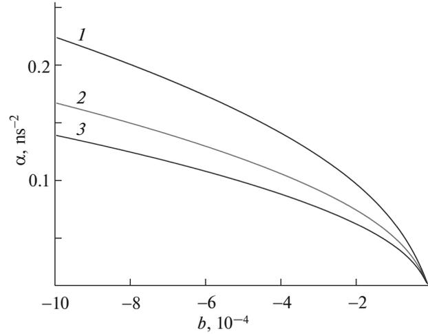
**Fig. 4.** Pulse chirp as a function of modulation depth  $b$  at  $z = 1 \text{ cm}$  for  $D_z = (0.5, 0.9, 1.3) \times 10^{-21} \text{ s}^2/\text{m}$  (curves 1–3, respectively).
