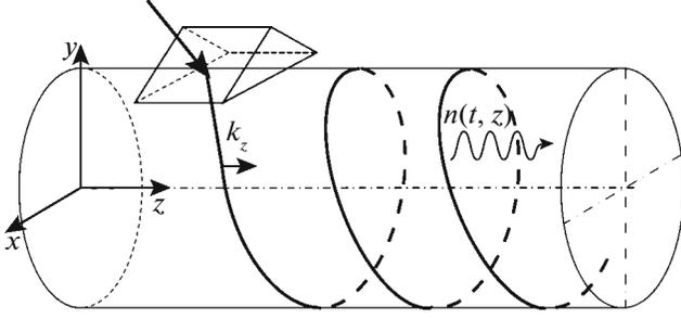
**Fig. 1.** Prism-coupling of a ray into a cylindrical optical waveguide and its trajectory of WGM type [21].
