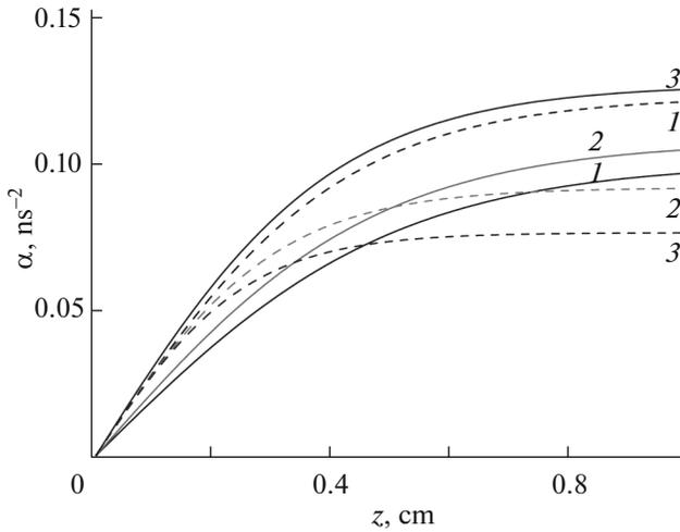
**Fig. 3.** The dependence of the TRIW-induced chirp on optical-waveguide length at  $b = -3 \times 10^{-4}$  and  $D_z = (0.5, 0.9, 1.3) \times 10^{-21} \text{ s}^2/\text{m}$  (solid lines 1–3, respectively); at  $D_z = 1 \times 10^{-21} \text{ s}^2/\text{m}$  and  $b = (-2, -2.3, -3.2) \times 10^{-4}$  (dashed lines 1–3, respectively).
