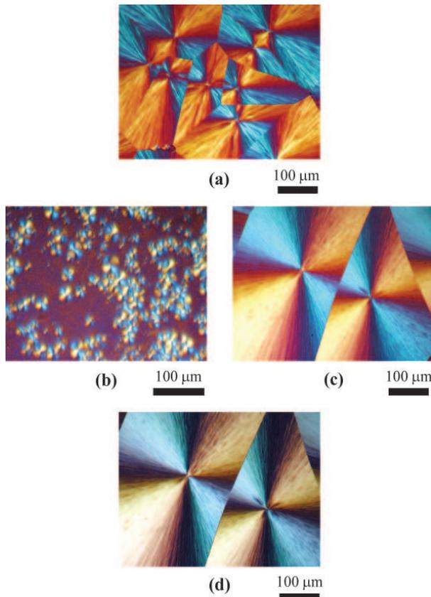
**Fig. 9.** Polarized-light micrographs of (a) 24PLLA homopolymer crystallized isothermally at 130 °C until saturation; (b) L<sub>55</sub>C<sub>45</sub> film quenched from the melt; (c) L<sub>55</sub>C<sub>45</sub> film crystallized isothermally at 130 °C until saturation; (d) same sample as in (c) after PCL crystallization at 40 °C.
