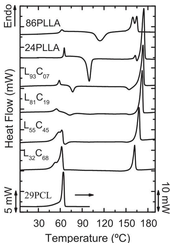
**Fig. 7.** DSC first heating scans from  $-20^{\circ}\text{C}$  at  $10^{\circ}\text{C}/\text{min}$  of compression-moulded films of PLLA-*b*-PCL diblock copolymers and corresponding homopolymers.
