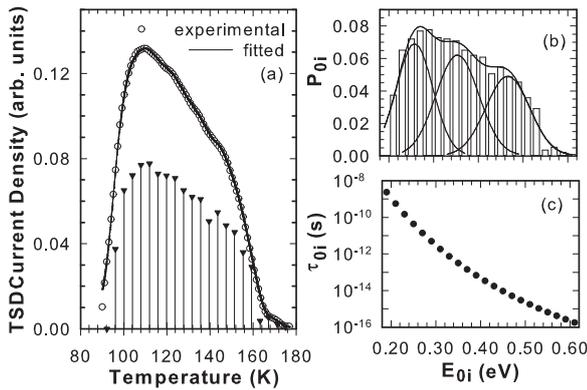
**Fig. 4.** Simulated annealing direct signal analysis of the low-temperature modes of the 55/45 PLLA-*b*-PCL block copolymer: (a) TSDC trace and positions of the Debye modes. (b) Energy histogram of the contributions to the total polarization. (c) Variation of the pre-exponential Arrhenius factor as a function of the activation energy of each Debye mode.
