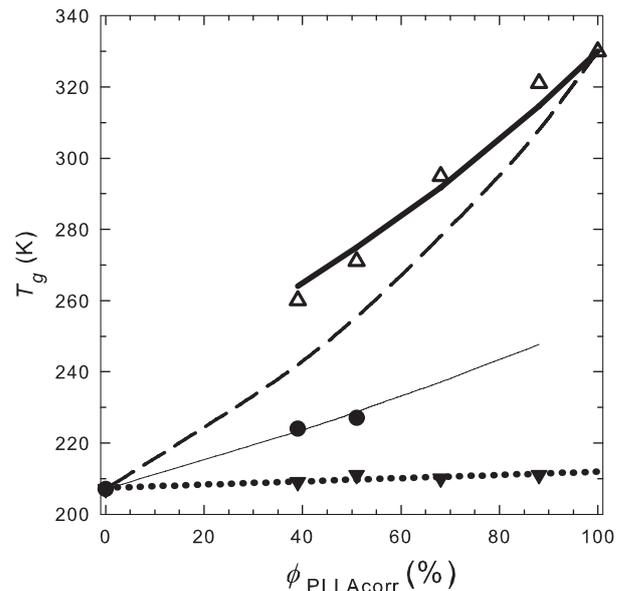
**Fig. 6.**  $T_g$ 's compositional variation: of the bulk (Fox dependence) (---); of the experimental effective  $T_g$ 's:  $T_g^{\text{eff}}_{\text{PLLA}}$  ( $\triangle$ );  $T_g^{\text{eff}}_{\text{PCL}}$  ( $\blacktriangledown$ ) and ( $\bullet$ ). Best fits: for  $\phi_s_{\text{PLLA}} = 31\%$  (thick solid line), for  $\phi_s_{\text{PCL}} = 100\%$  ( $\bullet\bullet\bullet\bullet$ ), for  $\phi_s_{\text{PCL}} = 50\%$  (thin solid line).
