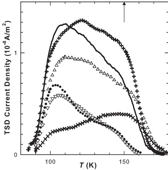
**Fig. 3.** Low-temperature TSDC spectra for the diblock copolymers PLLA-*b*-PCL for various bulk compositions;  $T_p = 150$  K. +: 0/100;  $\Delta$ : 32/68; —: 55/45;  $\nabla$ : 81/19;  $\bullet$ : 93/07;  $\times$ : 100/0.
