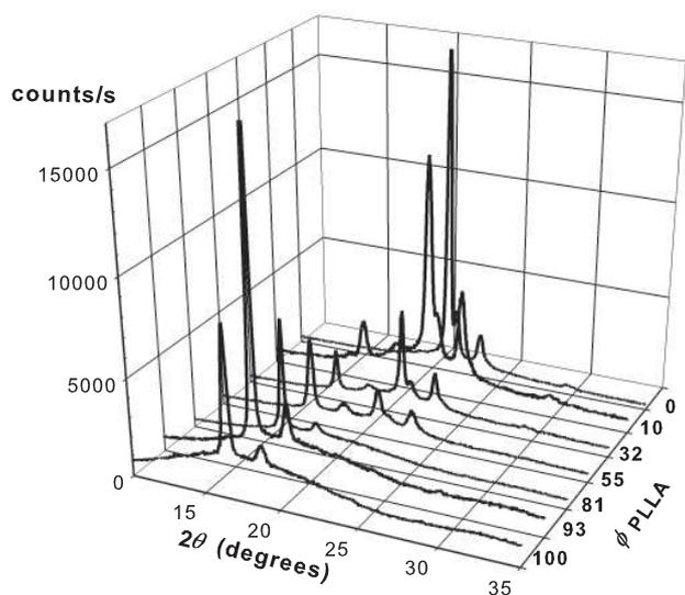
**Fig. 1.** WAXS patterns ( $\text{Cu } \lambda K\alpha$ ) at room temperature for PLLA-*b*-PCL copolymers with compositions from 100% PLLA (front) to 100% PCL (back).
