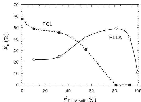
**Fig. 2.** Variation of crystallinity degrees with bulk composition of the two components of the diblock copolymer PLLA-*b*-PCL.
