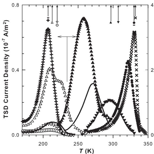
**Fig. 5.** High-temperature TSDC spectra for the diblock copolymers PLLA-*b*-PCL for various bulk compositions and polarization temperatures; +: 0/100;  $\triangle$ ,  $\blacktriangle$ : 32/68; —: 55/45;  $\nabla$ ,  $\blacktriangledown$ : 81/19;  $\circ$ ,  $\bullet$ : 93/07;  $\times$ : 100/0. Left scale for open symbols, right scale for filled symbols. The polarization temperatures are shown by vertical arrows.
