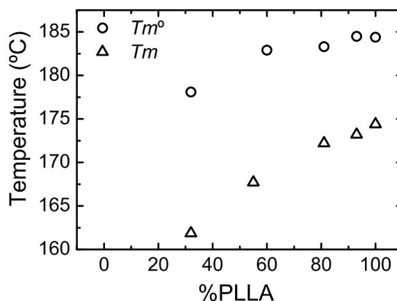
**Fig. 8.** Apparent melting temperatures obtained from Figure 7 and equilibrium melting temperatures ( $T_m^0$ ) for PLLA-*b*-PCL diblock copolymers as a function of the bulk composition.
