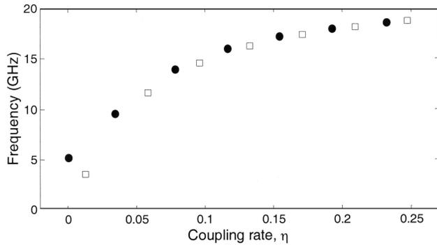
Fig. 4. Frequency of periodic solutions versus coupling rate as obtained numerically (circles) from Eqs. (1) and (2) and analytically (squares) from Eqs. (5)–(7).
