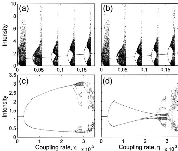
Fig. 1. Bifurcation diagrams of the optical power emitted by (a), (c) laser 1 and (b), (d) laser 2. (c), (d) Enlarged views of (a) and (b), respectively. The coupling rate is the bifurcation parameter.
