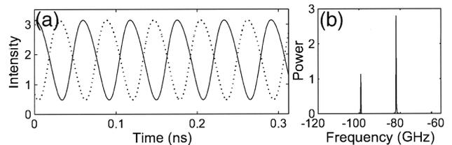
Fig. 3. (a) Time traces of the output of laser 1 (solid curve) and laser 2 (dotted curve). (b) Optical spectrum of laser 1. The coupling strength is  $\eta = 0.16$ .
