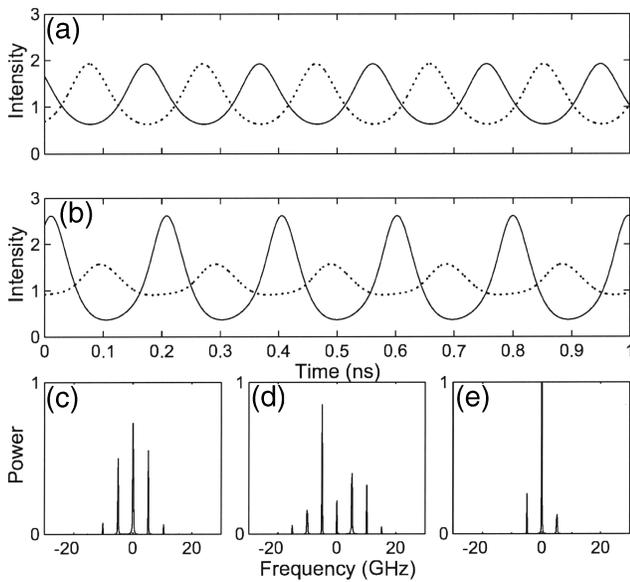
Fig. 2. (a), (b) Time traces of the outputs of laser 1 (solid curve) and laser 2 (dotted curve) for  $\eta = 5 \times 10^{-4}$  and  $\eta = 1.5 \times 10^{-3}$ , respectively. (c) Optical spectrum of laser 1 for  $\eta = 5 \times 10^{-4}$ . (d), (e) Optical spectra of laser 1 and laser 2, respectively, for  $\eta = 1.5 \times 10^{-3}$ .
