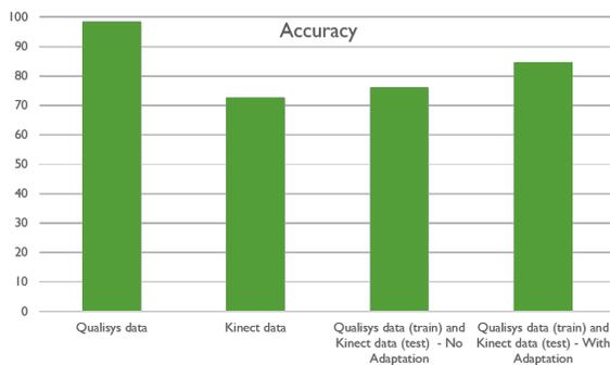
**Figure 11:** Comparison of recognition accuracy before and after adaptation
