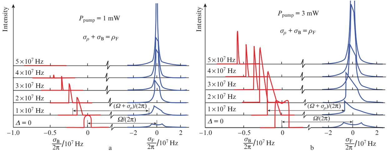
**Figure 4.** Dependences of the intensities of the forward and backward waves on the corresponding detunings  $\sigma_F$  and  $\sigma_B$  for various  $\Delta = (\Omega_B - \Omega)/(2\pi)$  and pump powers of (a) 1 and (b) 3 mW. Pay attention to the difference in scales for  $\sigma_F$  and  $\sigma_B$ .
