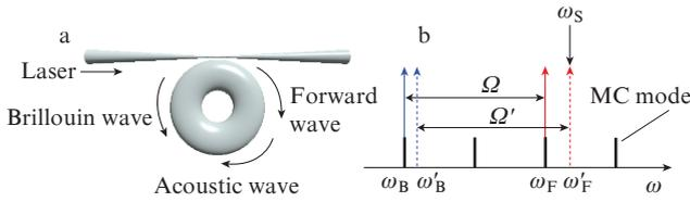
**Figure 1.** Schemes for (a) Brillouin lasing in the microcavity and (b) tuning the frequencies of the forward, backward, and acoustic waves when detuning the pump frequency from the frequency of the microcavity mode.
