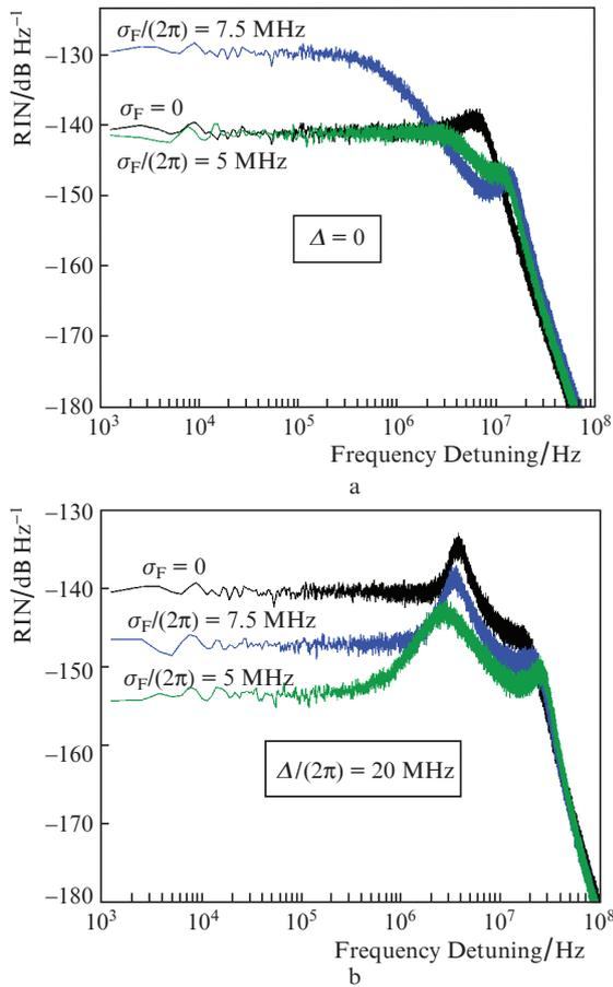
**Figure 5.** Results of numerical simulation. The spectral density of the relative noise intensity (RIN) of the Brillouin signal in the MC at different pump detunings (a) in the case of the coincidence of the Brillouin shift and the intermode spacing and (b) at the detuning  $(\Omega_B - \Omega)/(2\pi) = 20$  MHz.
