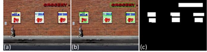
Fig. 2. Result of text detection. (a) Input image, (b) Text detection (green bounding-boxes), and (c) Binary text masks.
