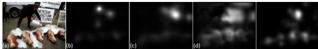
Fig. 5. Result where DNN-base models is less good than bottom-up models. (a) Input image, (b) Result of SAM-ResNet, (c) Result of Salicon, (d) Result of our model and (e) Eye tracking map.
