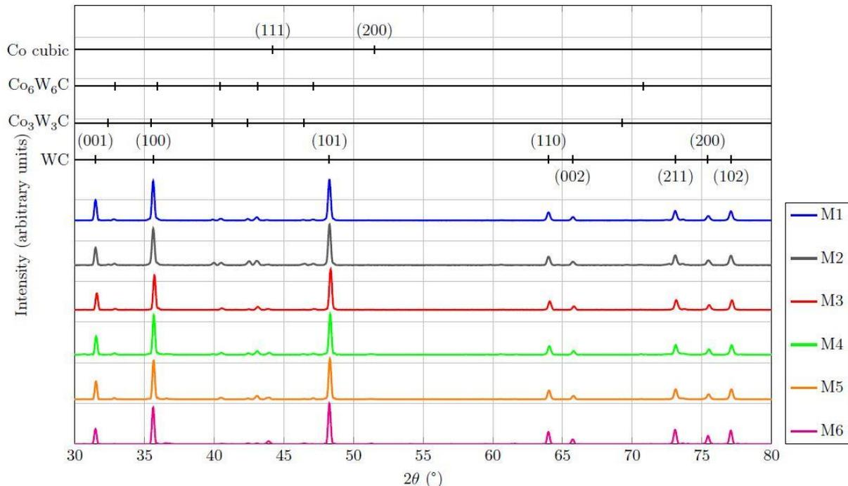
**Figure 1 – XRD patterns of the sintered samples**
