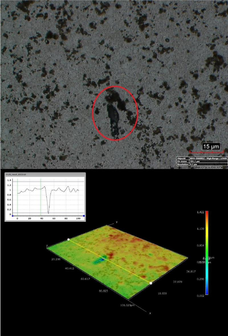
Figure 4 - Microstructure and 3D imaging of the 100 wt% recycled powder (M1)
