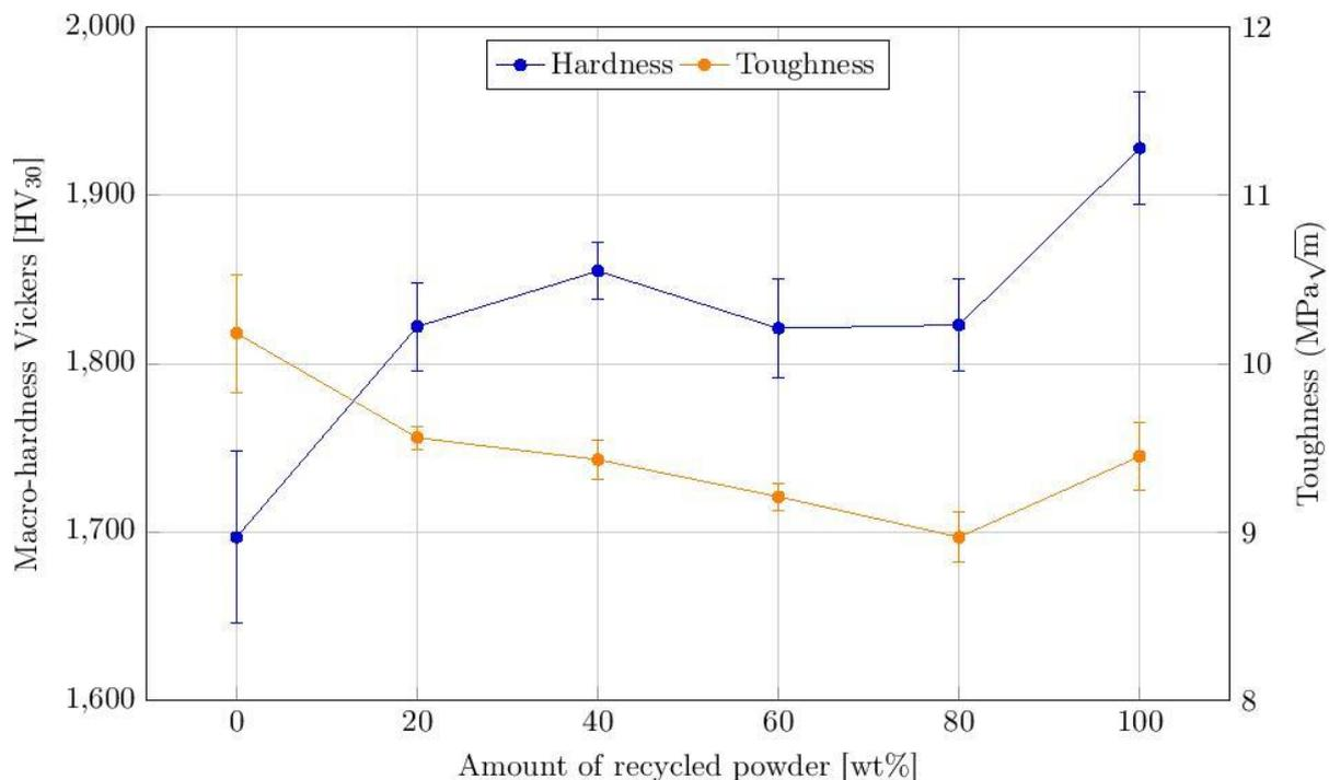
Figure 2 - Mechanical properties of the sintered samples (macro-hardness Vickers and Palmqvist toughness)
