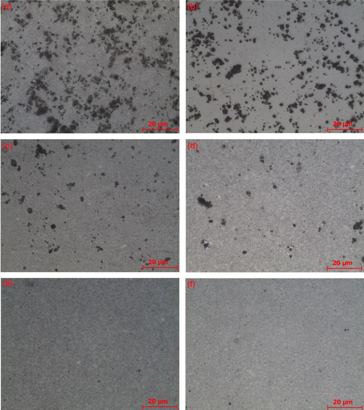
Figure 3 - Microstructures as function of the amount of recycled powder: (a) 100%, (b) 80%, (c) 60%, (d) 40%, (e) 20%, (f) 0%; etched by Murakami reagent (x 500)
