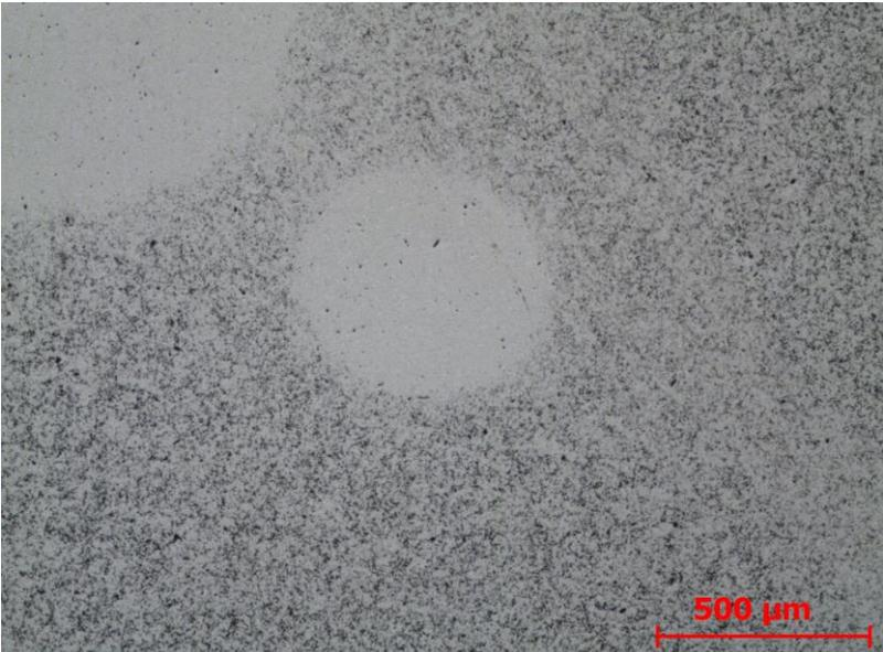
Figure 5 - Sample M1 (100 wt% recycled powder): presence of areas without defects
