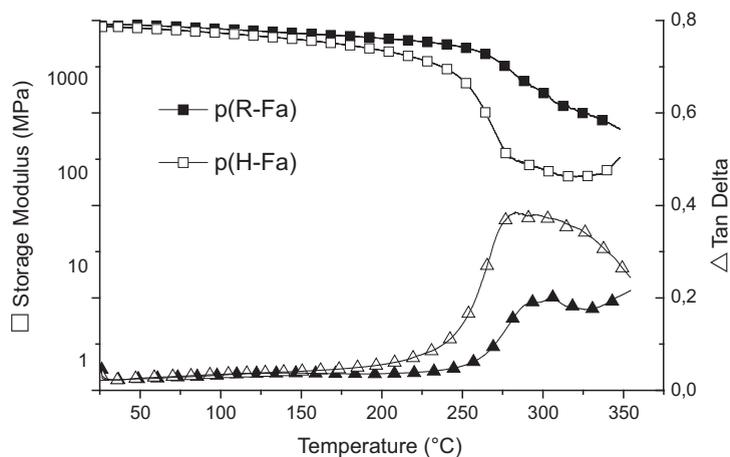
Fig. 7. Evolution of the thermomechanical behavior of p(R-Fa) (closed symbols) and p(H-Fa) (open symbols). Frequency: 1 Hz, Temp ramp rate: 3 °C min<sup>-1</sup>.
