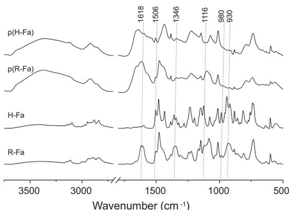
Fig. 6. FTIR spectra of R-Fa and H-Fa precursors and their respective crosslinked polymers p(R-Fa) and p(H-Fa).
