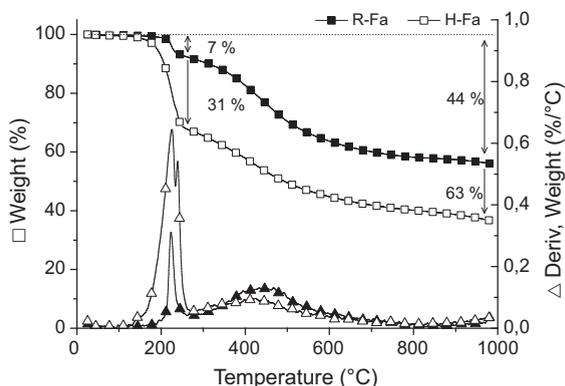
Fig. 5. TGA profiles of R-Fa and H-Fa precursors under nitrogen.
