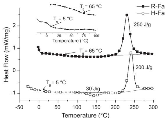
Fig. 4. DSC thermograms of R-Fa and H-Fa precursors. Inset: zoom on the precursors glass transition temperatures.
