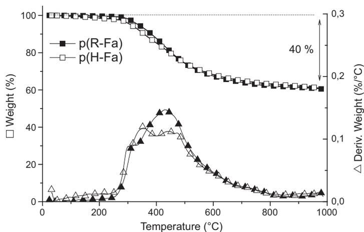
Fig. 8. TGA profiles of p(R-Fa) and p(H-Fa) obtained under nitrogen at 10 °C min<sup>-1</sup>.
