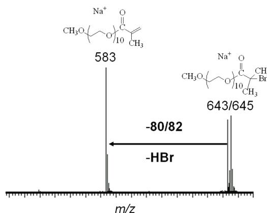
**Fig. 4.** CID mass spectrum of  $m/z$  643/645 at 25 eV.
