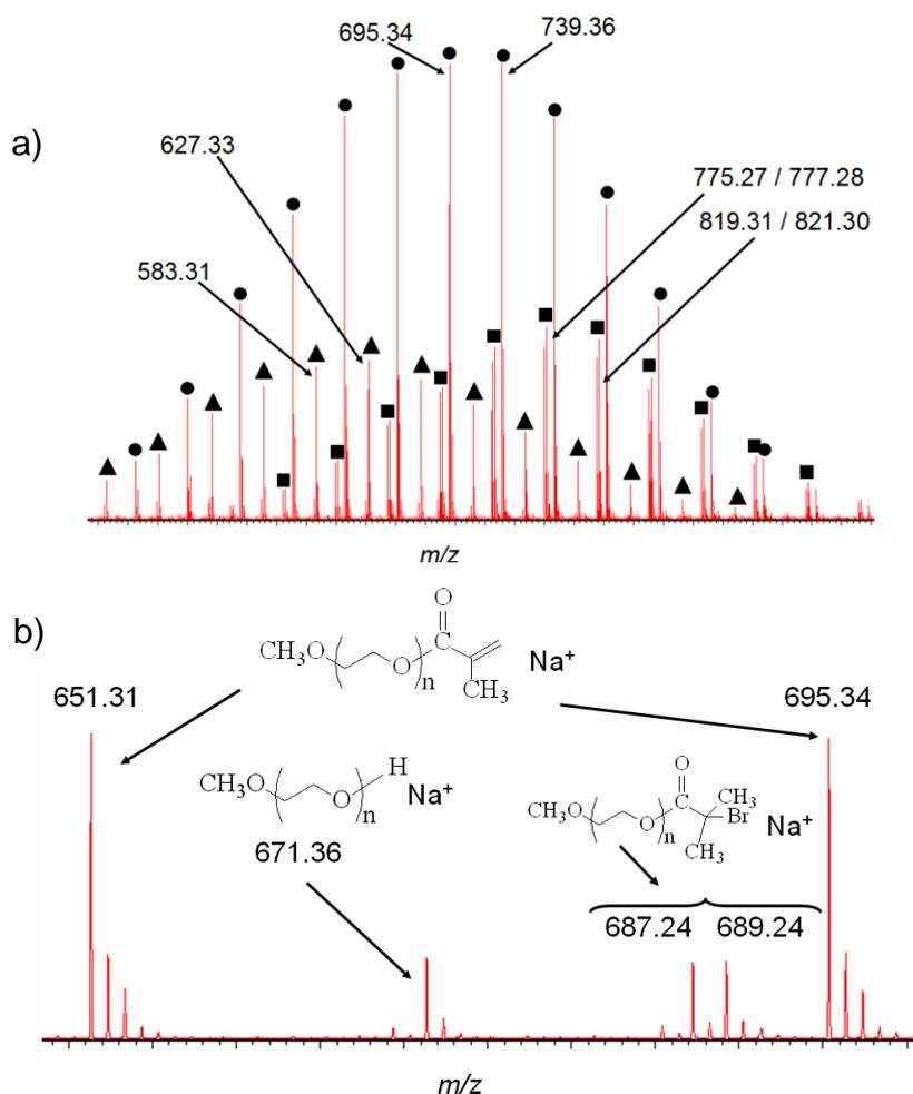
**Fig. 2.** MALDI-ToF analysis of PEOBr ( $M_n$  SEC  $700 \text{ g.mol}^{-1}$ ) using  $\alpha$ -cyano-4-hydroxycinnamic acid as the matrix and a laser fluence of  $350 \text{ J.m}^{-2}$  : (a) global mass spectrum and (b) partial view from  $m/z$  650 to 700.
