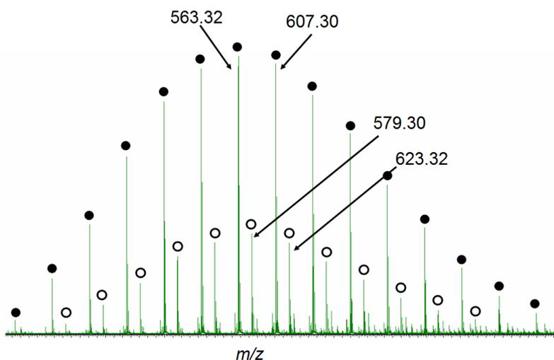
**Fig. 1.** PEOMA MALDI-ToF analysis ( $M_n$  NMR  $530 \text{ g.mol}^{-1}$ ) using  $\alpha$ -cyano-4-hydroxycinnamic acid as the matrix and a laser fluence of  $350 \text{ J.m}^{-2}$  : global mass spectrum.
