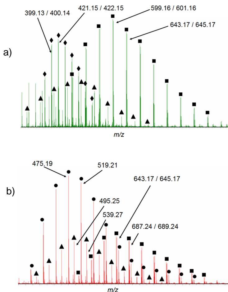
**Fig. 3.** ESI-ToF analysis of PEOBr ( $M_n$  SEC 700  $\text{g}\cdot\text{mol}^{-1}$ ) : (a) global mass spectrum recorded at 20 V and (b) recorded at 70 V cone voltage.
