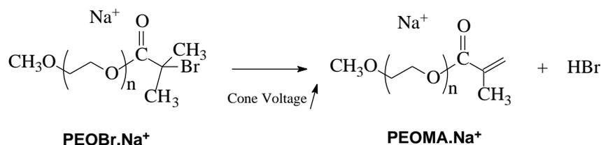
**Scheme 2.** In Source collision-induced HBr elimination from  $\text{Na}^+$ -cationized PEOBr.
