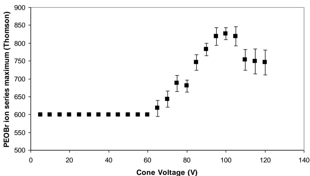
**Fig. 5.** ESI-ToF analysis of PEOBr ( $M_n$  SEC 700  $g.mol^{-1}$ ): influence of the cone voltage (V) on the PEOBr ion series maximum.
