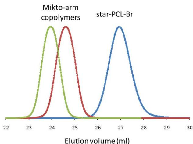
**FIGURE 3** SEC traces of the star-shaped PCL-Br macroinitiator ( $M_n = 2700 \text{ g mol}^{-1}$ ; blue curve) and two corresponding mikto-arm copolymers obtained after MAIGP ATRP (red curve = entry 1, Table 2; green curve = entry 2, Table 2).
