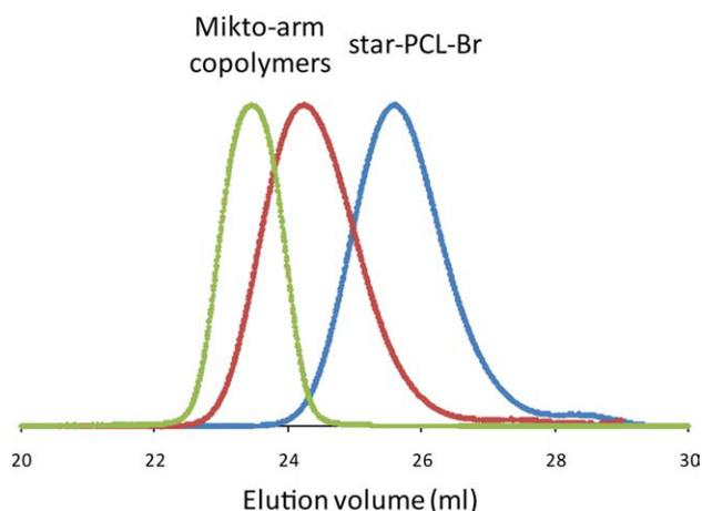
**FIGURE 4** SEC traces of the initial three-arm star-shaped PCL macroinitiator ( $M_n = 6300 \text{ g mol}^{-1}$ ; blue curve) and two mikto-arm copolymers obtained via ATRP (red curve = entry 3, Table 2; green curve = entry 4, Table 2).
