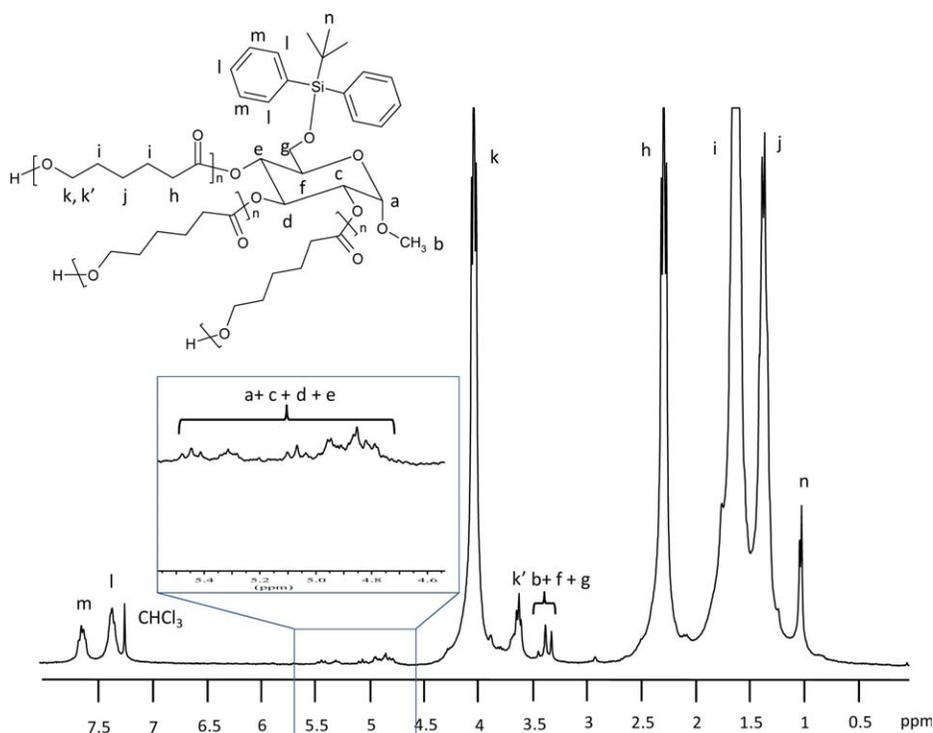
**FIGURE 1**  $^1\text{H}$  NMR spectrum of three-arm star-shaped PCL in  $\text{CDCl}_3$  (entry 2, Table 1) (signal  $k'$  is attributed to the  $-\text{CH}_2-\text{OH}$  end-group). [Color figure can be viewed in the online issue, which is available at [www.interscience.wiley.com](http://www.interscience.wiley.com).]
