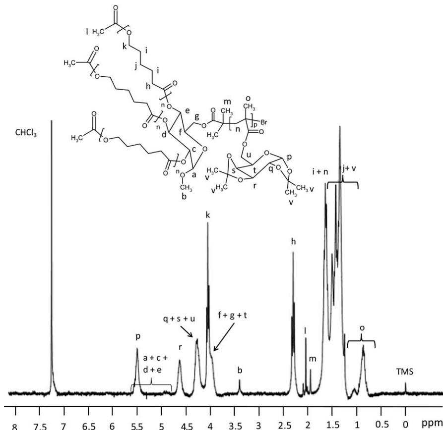
**FIGURE 2** <sup>1</sup>H NMR spectrum (CDCl<sub>3</sub>) of a mikto-arm copolymer based on three-arm star-shaped PCL and MAIGP (see entry 2, Table 2).
