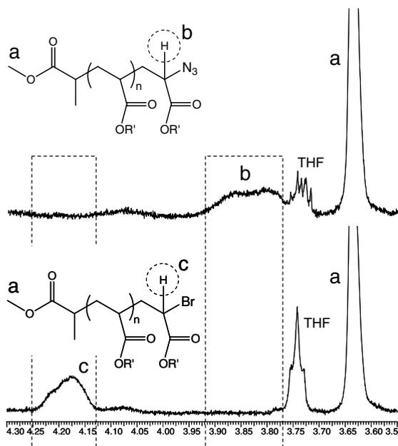
Fig. 4. Transformation of PiBA-Br into PiBA-N<sub>3</sub> (Table 2, entry 9), as evidenced by <sup>1</sup>H NMR (CDCl<sub>3</sub>, 500 MHz).
