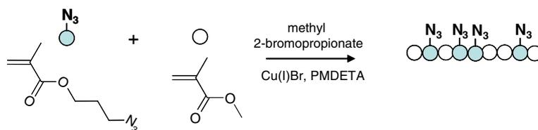
Fig. 5. Schematic depiction of the copolymerization of MMA and AzMA to yield a random copolymer containing multiple azide functionalities.
