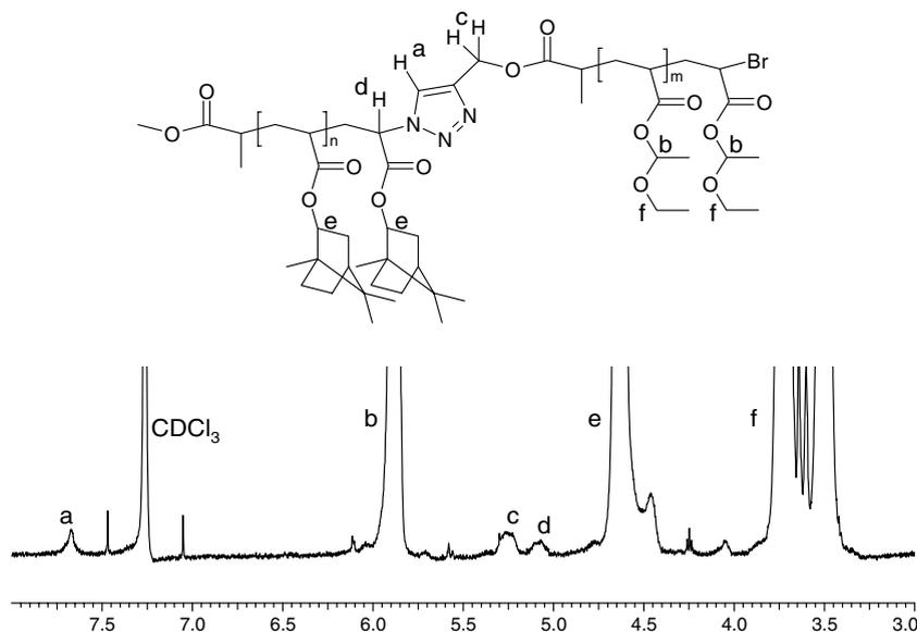
Fig. 7.  $^1\text{H}$  NMR spectrum of the product of “click” coupling reaction (Table 4, entry 12) of  $\text{PiBA-N}_3$  (Table 2, entry 10) and  $\text{PEEA-}\equiv$  (Table 1, entry 6) to yield a poly( $i\text{BA-}b\text{-EEA}$ ) block copolymer (in  $\text{CDCl}_3$ , 500 MHz).
