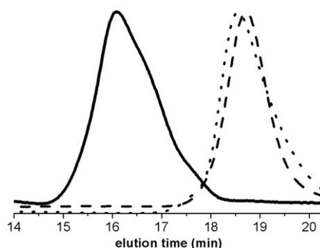
Fig. 9. GPC traces of “click” coupling reaction (Table 5, entry 14) of a poly( $\text{MMA-}co\text{-AzMA}$ ) copolymer (Table 3, entry 11, dotted line) and a  $\text{PEEA-}\equiv$  polymer (Table 1, entry 8, dashed line), before the coupling reaction, and after the “click” reaction (solid line, after purification by preparative GPC).
