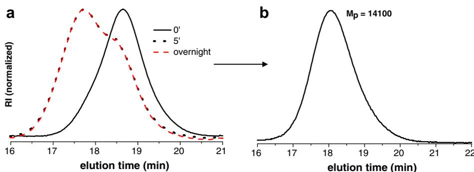
Fig. 6. (a) GPC traces of “click” coupling reaction (Table 4, entry 12) of PiBA-N<sub>3</sub> and a PEEA-≡ polymer, before the coupling reaction (0', mixture of start products), after 5 min (5'), and overnight. (b) GPC trace of the same “click” coupling reaction (Table 4, entry 12) after removal of the excess PEEA-≡ by selective precipitation in methanol.
