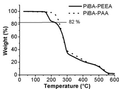
Fig. 8. TGA analysis of the “click” coupled poly( $i\text{BA-}b\text{-EEA}$ ) block copolymer before (solid line) and after deprotection (dotted line) by a heating process at  $80\text{ }^\circ\text{C}$  during 24 h (Table 4, entry 12). Heating rate:  $10\text{ }^\circ\text{C}/\text{min}$ ; air atmosphere.
