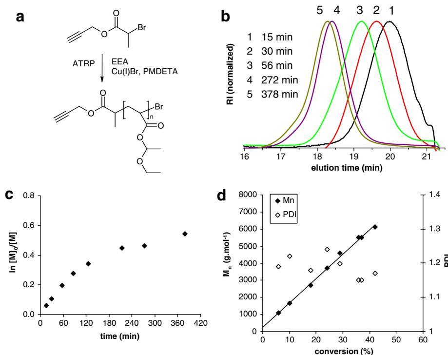
Fig. 2. ATRP of EEA using an alkyne-containing initiator (Table 1, entry 4). (a) schematic depiction, (b) GPC analysis, (c) first order kinetic plot, (d) increase of  $M_n$  and evolution of PDI as a function of conversion. (With trend line in graph (d)).
