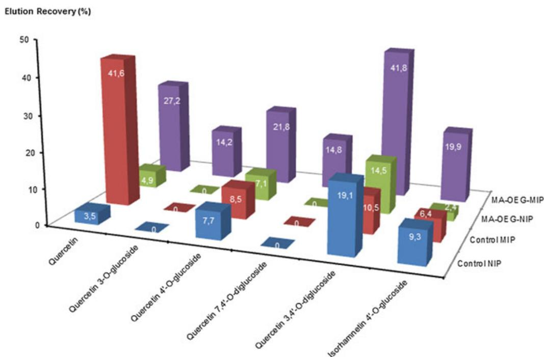
**Figure 4.** Recoveries measured on solid phase extraction (SPE) columns packed with Control NIP, Control MIP, MA-OEG-NIP and MA-OEG-MIP. Sample solution: *Allium cepa* raw methanol/water extract (924 µg/800 mg polymer). [Colour figure can be viewed at wileyonlinelibrary.com]
