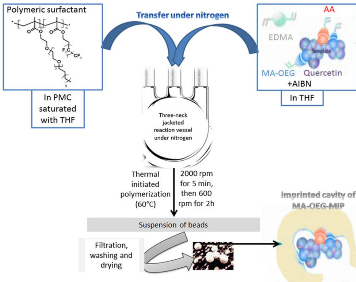
**Figure 2.** Schematic graph of the preparation of MA-OEG-MIP. [Colour figure can be viewed at [wileyonlinelibrary.com](http://wileyonlinelibrary.com)]
