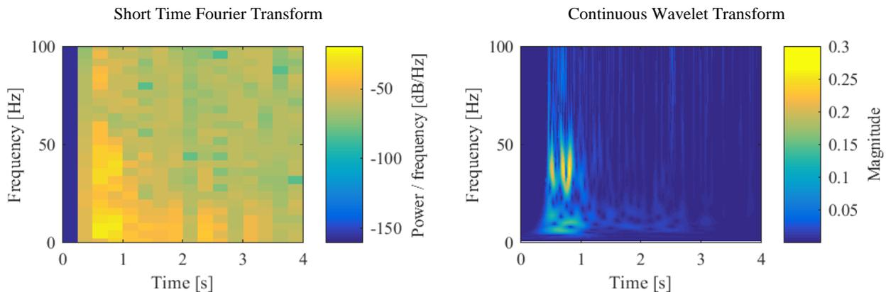
Figure 7: Comparison of the time-frequency analysis of the vertical component of the ground vibration record BL\_01 using (a) the Short Time Fourier Transform ( $\delta t = 0.25 s / \Delta f = 4.00 Hz$ ), and (b) the Continuous Wavelet Transform ( $N_{oct} = 10, N_{voi} = 10$ ).
