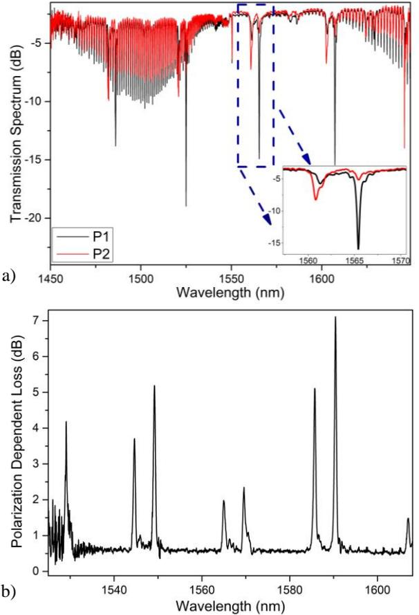
Fig. 3 a) Transmitted spectrum of a 10<sup>th</sup>-order 10° TFBG in the wavelength range 1450–1650 nm. Inset: Orthogonal polarization dependence of the leaky mode resonance closest to the Bragg peak. b) Polarization Dependent Loss of the 10th-order 10° TFBG in the wavelength range 1520–1610nm measured by LUNA OVA.
