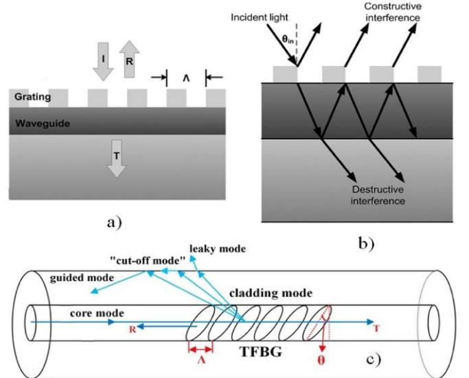
Fig. 1 a) Schematic view of a leaky/guided-mode resonance, b) Leaky coupling at resonance according to the model in ref. [41], c) Schematic of TFBG geometry. Coupling from the core mode to numerous cladding modes where R (reflection), T (transmission),  $\Lambda$  (grating period) and  $\theta$  (Tilt angle) are shown.
