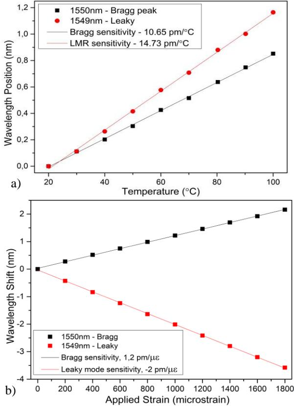
Fig. 4 Comparative measurement of Bragg mode with the closest leaky mode resonance in: a) Temperature, b) Axial Strain.
