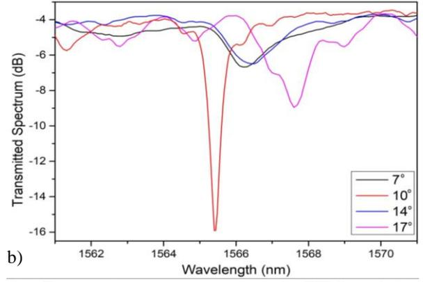
Fig. 2 a) Transmission spectrum of tenth order TFBGs at different tilt angles. For all cases the Bragg peak was selected at 1550nm, b) Comparison between different tilt angles with respect to transmission loss.
