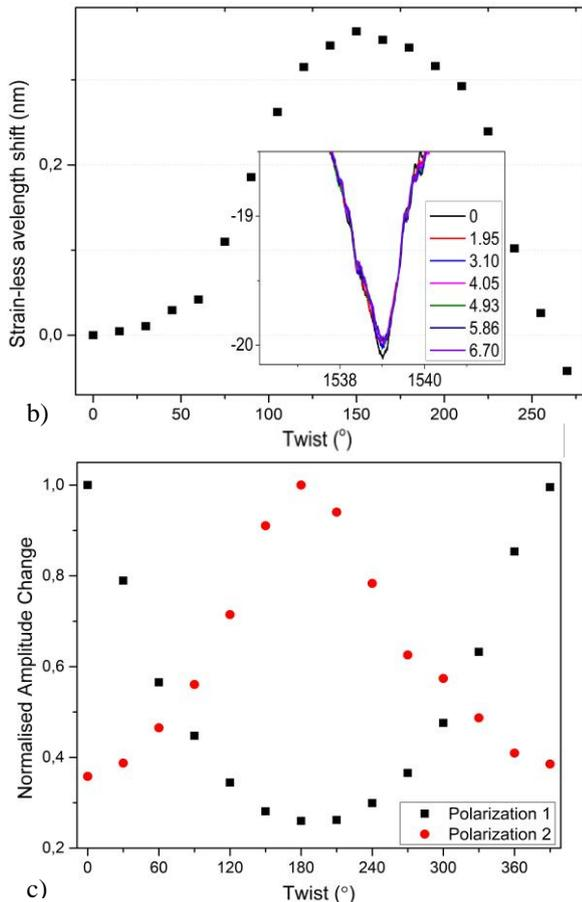
Fig. 5 Torsion behavior of a leaky mode resonance. a) Wavelength shift during twisting and from strain during the measurement. Inset: Actual mode shift and power de-coupling for the first 90 degrees, b) Pure torsion sensitivity of the LMR. Inset: Bend insensitivity per curvature change c) Normalized amplitude shift between the two polarizations of an LMR.
