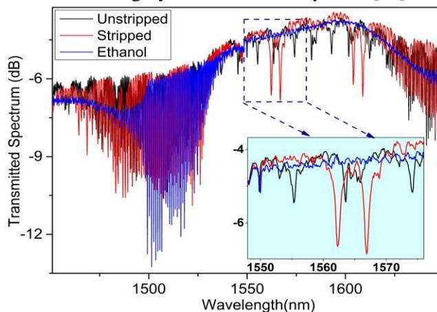
Fig. 7 Transmitted spectrum of 10<sup>th</sup> order 10° TFBG, stripped in air and dipped in ethanol. In ethanol, leaky modes vanish.
