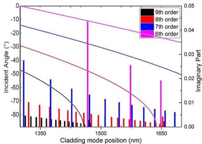
Fig. 6 Fimmwave simulation of the higher order mode location (bar chart) for each individual order along with the Matlab simulation (curved lines) for a leaky waveguide coupling as calculated from equation 3.
