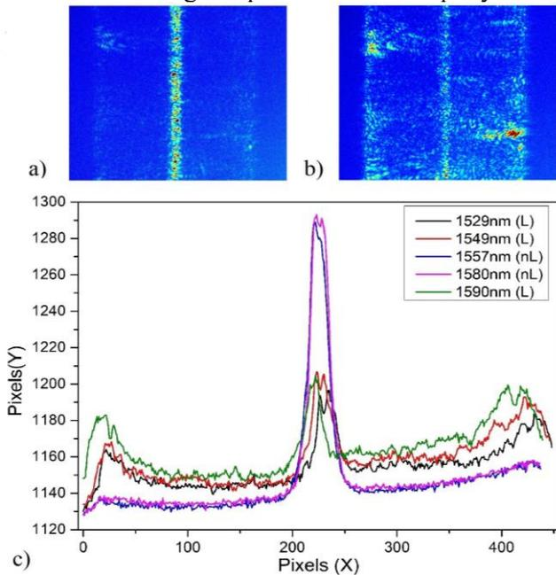
Fig. 8 Infrared camera image of the fiber core when light is launched using a tunable laser. a) Tuned to a wavelength with no LMR (nL). b) Tuned to a wavelength coincident with the LMR (L). c) Pixel intensity analysis showing the light distribution for a), b).
