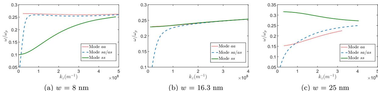
Figure 7: Dispersion at the center of the Brillouin zone for nanorod arrays of width (a)  $w = 8$  nm (b)  $w = 16.3$  nm (c)  $w = 25$  nm.
