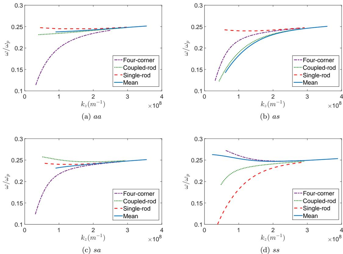
Figure 8: Comparison between the mean calculated with equation 2 and the three possible elementary excitations for the medium size nanorod array. (a) *aa* mode. (b) *as* mode. (c) *sa* mode. (d) *ss* mode.
