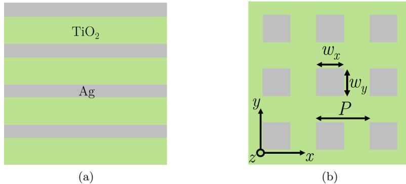
Figure 1: (a) Metamaterial consisting of periodic subwavelength layers of silver (Ag) and  $\text{TiO}_2$ . (b) Metamaterial consisting of an array of square or rectangular silver nanorods in a  $\text{TiO}_2$  host.  $w_x$  and  $w_y$  are the size of the nanorods in the  $x$  and  $y$  directions,  $P$  is the period of the array.
