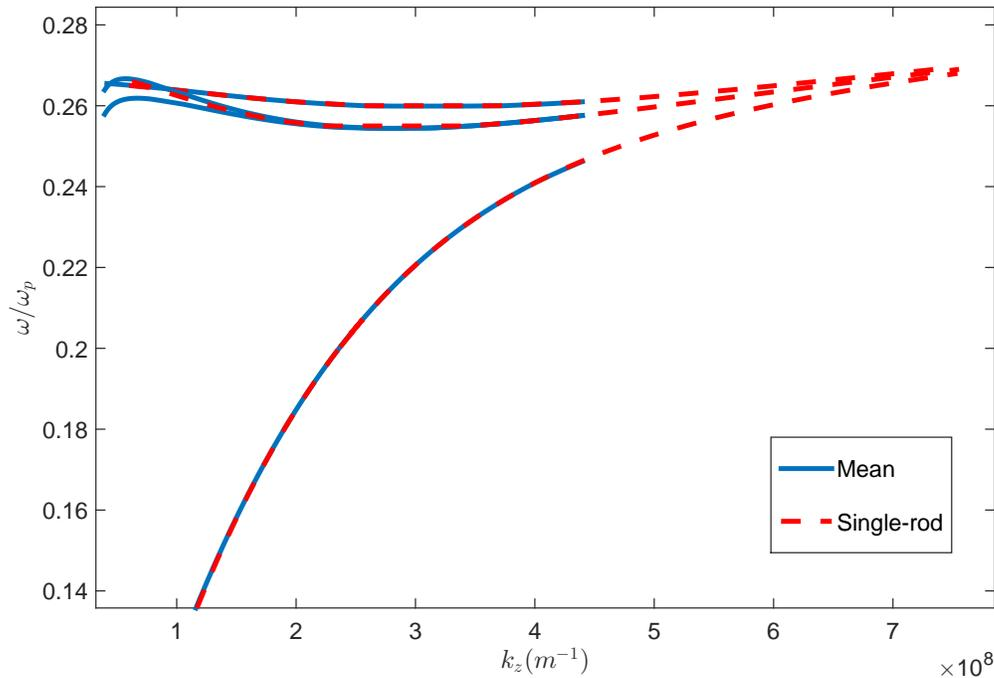
Figure 5: Comparison between the mean calculated with equation 2 and the single-rod excitation for the small nanorod array.
