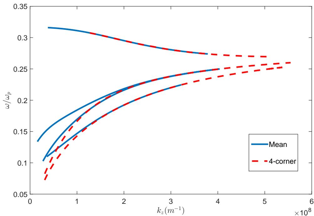
Figure 6: Comparison between the mean calculated with equation 2 and the four-corner excitation for the large nanorod array.
