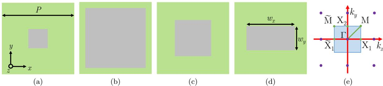
Figure 2: Single unit cell of the studied structures, the period in  $x$  and  $y$  direction is  $P = 30$  nm: array of square nanorods with width (a)  $w = 8$  nm, (b)  $w = 25$  nm, (c)  $w = 16.3$  nm. (d) Array of rectangular nanorods of width  $w_x = 20$  nm and  $w_y = 10$  nm. (e) Reciprocal lattice and first Brillouin zone (in light blue).
