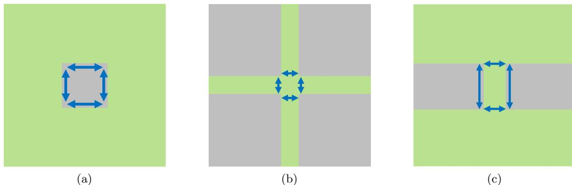
Figure 3: Elementary structures related to the arrays: (a) single rod in an infinite dielectric host. (b) Four metallic corners connected via dielectric medium. (c) Two coupled semi-infinite rods. Blue arrows indicate the principal ways of coupling between corners.
