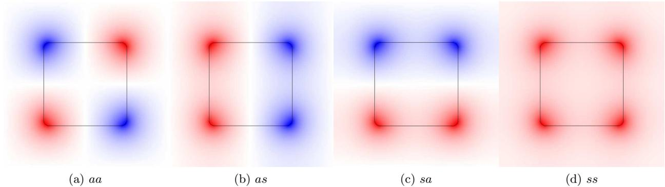
Figure 4: Component  $E_z$  of the electric field over a single unit cell for an array mode at the  $\Gamma$  point for  $w = 16.3$  nm at  $\lambda_0 = 700$  nm. (a)  $aa$  mode. (b)  $as$  mode. (c)  $sa$  mode. (d)  $ss$  mode.
