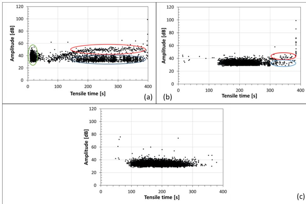
Figure 5. Recording of noise during tensile test of AA2024 alloy (a) in W state, (b) after 5 hours of natural aging, (c) after 24 hours of aging at 50°C
