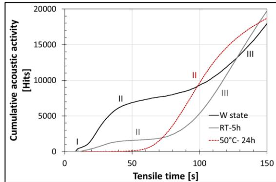
Figure 6. Evolution with aging treatment of acoustic activity of AA2024 alloy during tensile test
