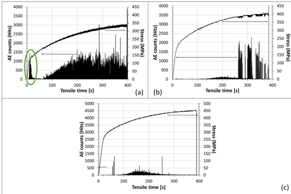
Figure 4. Tensile curves and recording of the acoustic emission during tensile test for AA2024 (a) in W state, (b) after 5 hours of aging at RT, (c) after 24 hours of aging at 50°C
