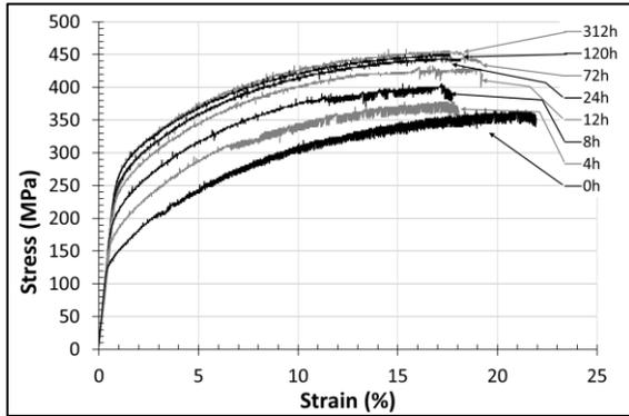
Figure 2. Stress-strain curves of AA2024 alloy after various times of natural aging treatment
