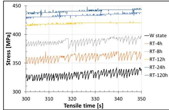
Figure 3. Magnified images of tensile curves of AA2024 alloy after various times of natural aging treatment
