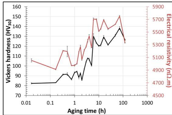
Figure1. Kinetic evolutions of hardness and electrical resistivity during natural aging treatment
