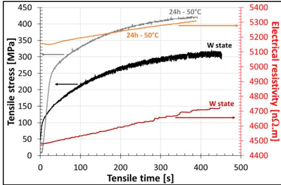
Figure 7. Evolution with tensile test of electrical resistivity of AA2024-W and after 24 hours of aging at 50°C
