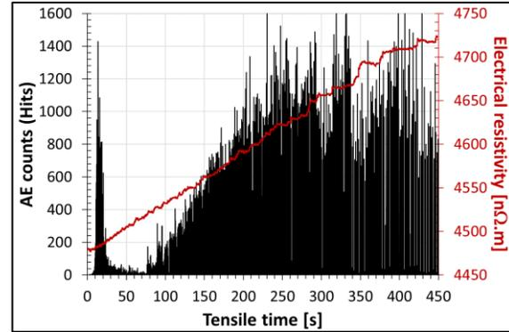
Figure 8. Evolution with tensile test of acoustic activity and electrical resistivity of AA2024-W
