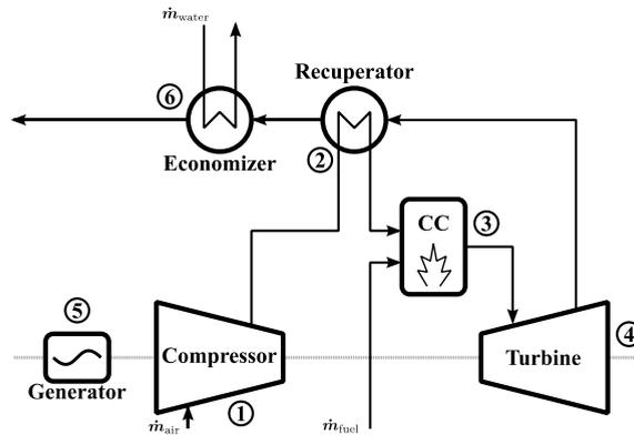
Figure 1: The Turbec T100 mGT, which is a typical recuperated mGT, was used as reference machine for the advanced humidified mGT cycles.
