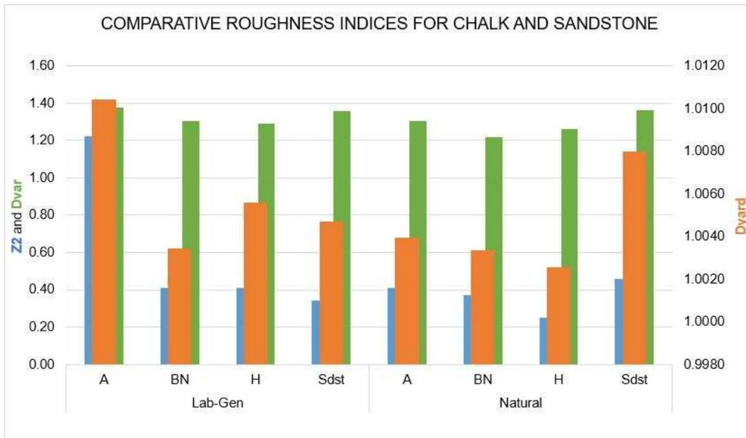
**Figure 1- Comparative roughness indices Z2, Dvar and Dyard for three chalks and a sandstone, natural fractures and lab-generated fractures.**
