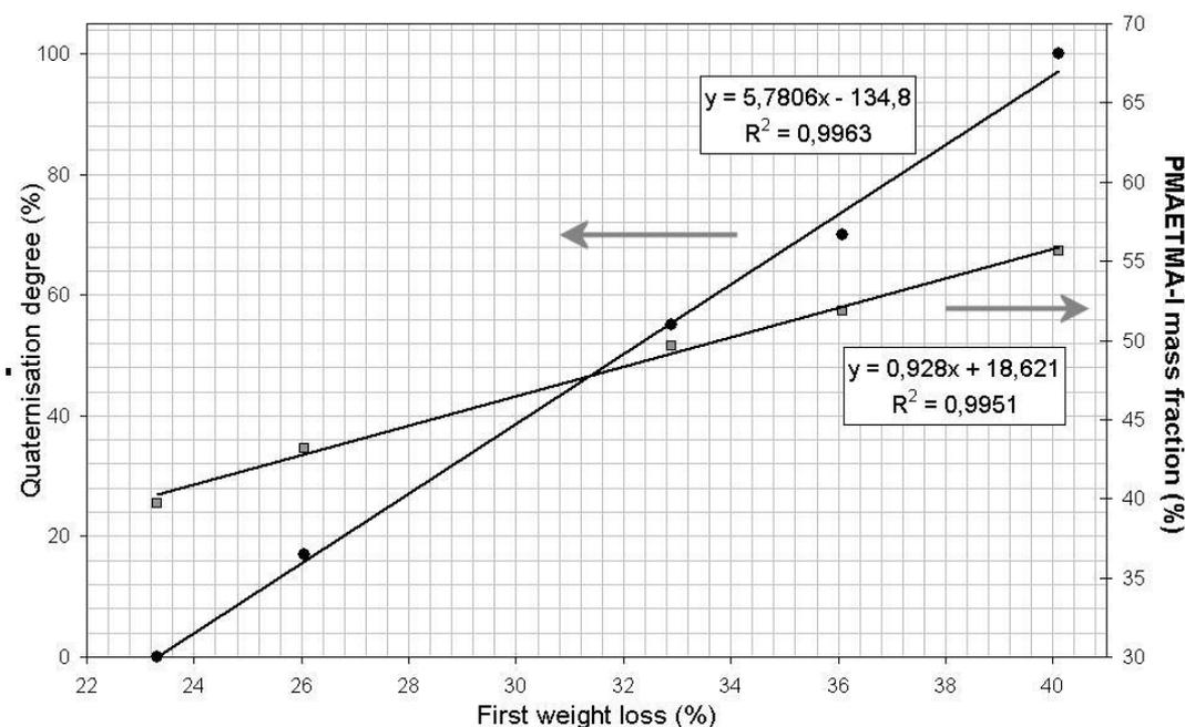
**Fig. 7.** Correlation between the degree of quaternization (DQ) and the mass fraction recorded at the first weight loss for PDMS-*b*-PMAETMA-I copolymers with different DQ values as determined by TGA.
