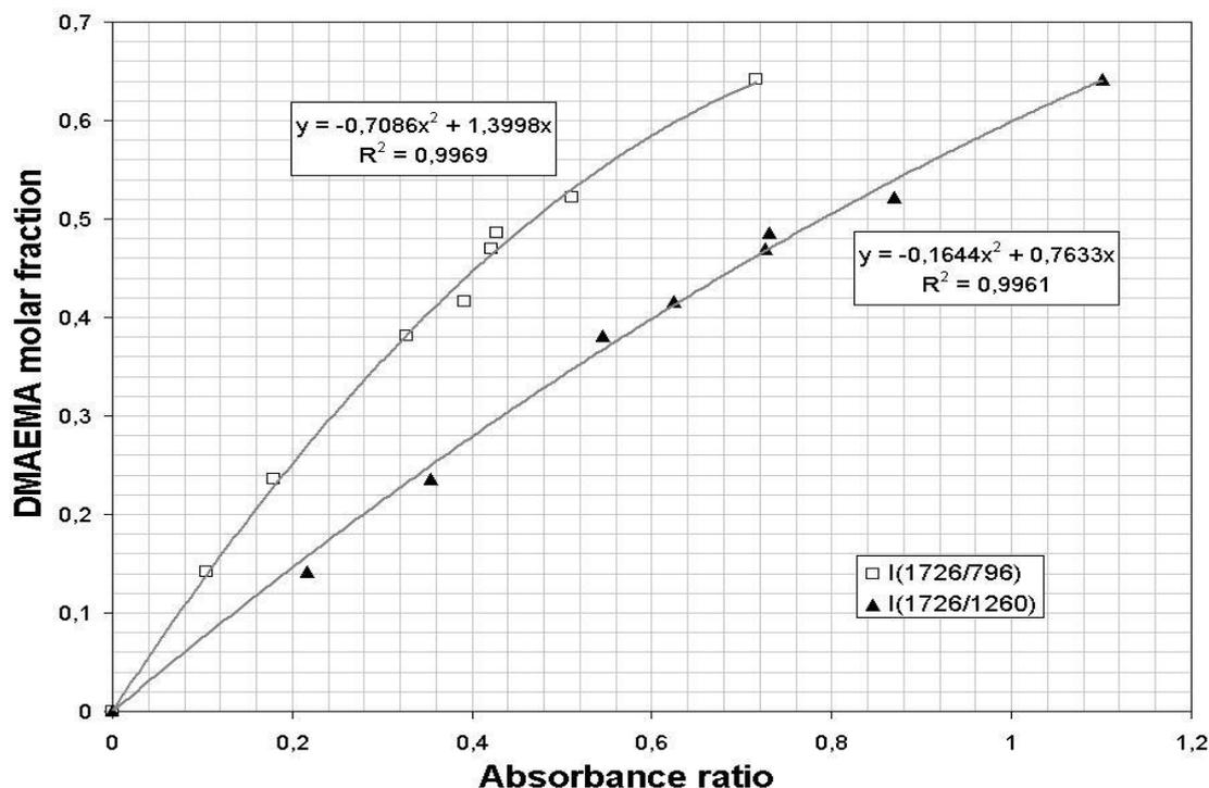
**Fig. 5.**  $^1\text{H}$  NMR/ATR-FTIR correlation curves as obtained for PDMS-*b*-PDMAEMA diblock copolymers of different DMAEMA molar fractions.
