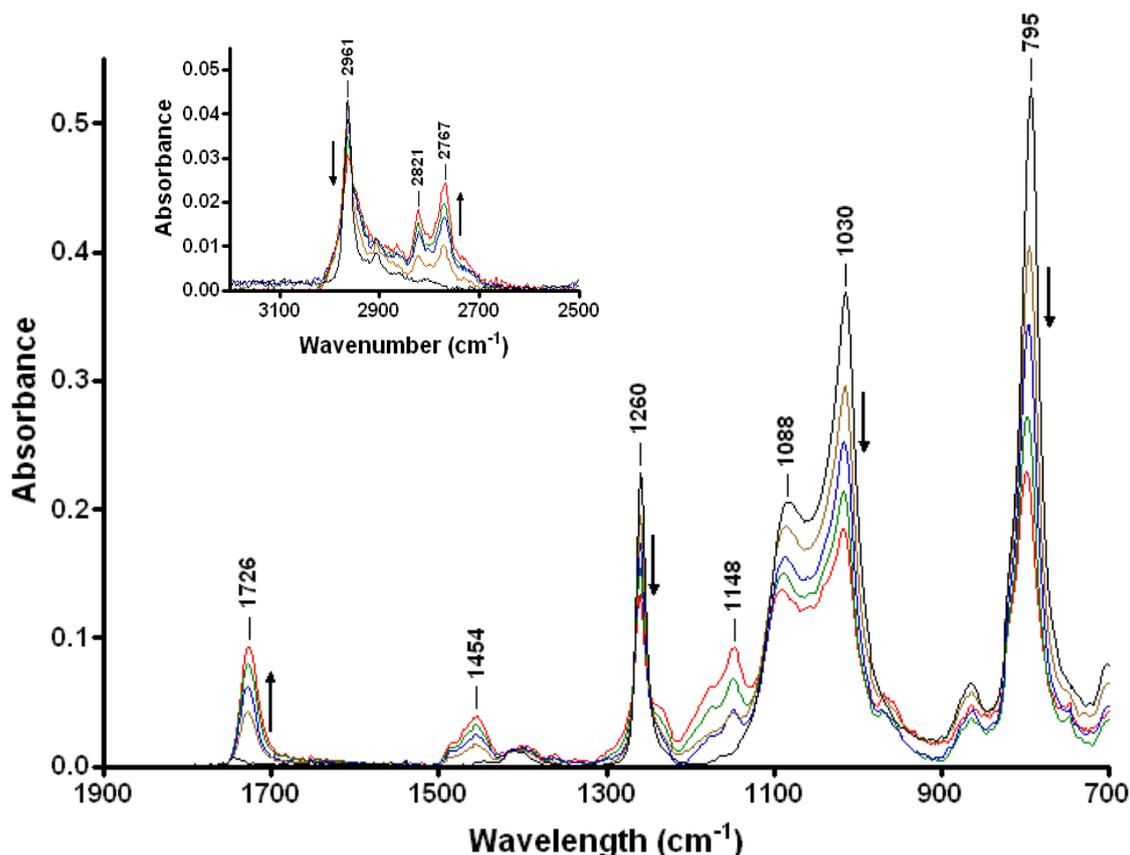
**Fig. 4.** ATR-FTIR spectra of  $\omega$ -bromo PDMS (black line) and a series of PDMS-*b*-PDMAEMA block copolymers with  $DP_{\text{PDMAEMA}}$  22 (brown line), 41 (blue line), 82 (green line) and 126 (red line). In the inset the absorbance between  $2500\text{ cm}^{-1}$  and  $3100\text{ cm}^{-1}$  is shown.
