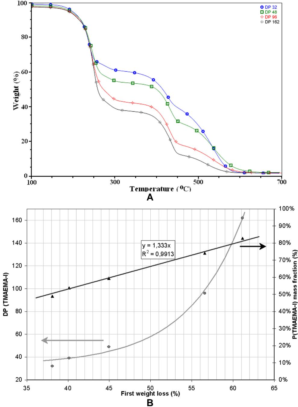
**Fig. 8.** TGA curves (A) and correlation between the degree of polymerization (DP) and the mass fraction on the first weight loss (B) for PDMS-*b*-PMAETMA-I copolymers with different PMAETMA-I block lengths.
