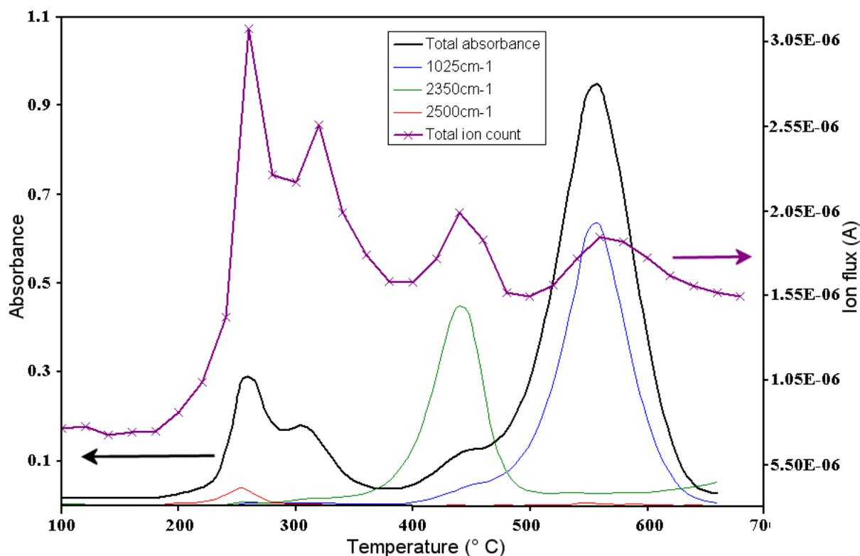
**Fig. 9.** Evolved gas analysis by ATR-co-FTIR/MS as obtained for Entry 10 (Table 3). Overlay of the total ion count by MS and total IR absorbance and those due to peaks at 2500 (Me<sub>3</sub>N<sup>+</sup>-H), 2350 (CO<sub>2</sub>) and 1025 cm<sup>-1</sup> (siloxane cyclo-oligomers).
