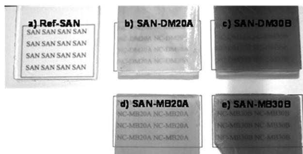
**Fig. 1** Optical transparency of SAN and SAN/clay nanocomposites on 3 mm-thick compression-molded samples. DM stands for direct-mixed and MB for masterbatch-mixed.
