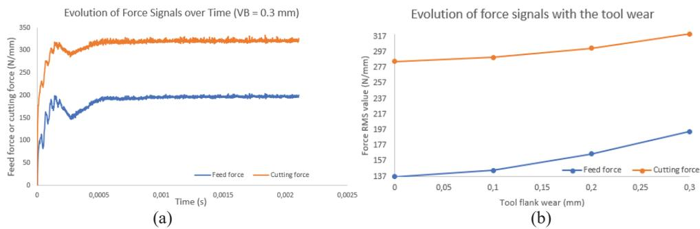
**FIGURE 3.** Evolution of the cutting and feed force numerically computed in the case of VB = 0.3 mm (a), and evolution of the cutting force and feed force for various phases of cutting tool flank wear (b).
