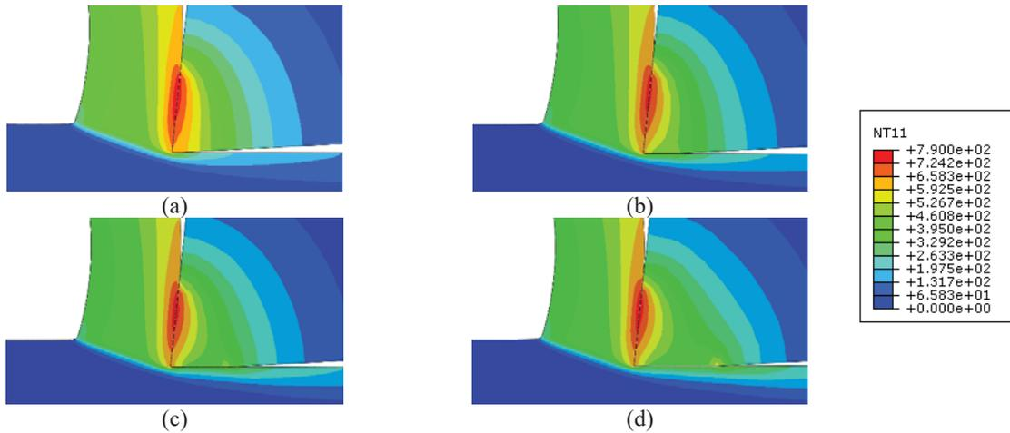
**FIGURE 2.** Temperature contour plot of the fresh tool geometry (a), and VB = 0.1 mm (b), 0.2 mm (c) and 0.3 mm (d). The colour scale, which is common to all diagrams, is provided.
