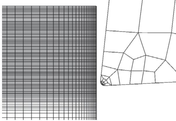
**FIGURE 1.** Model features at initial time on the fresh tool initial model. The depth of cut is  $0.1$  mm, with the workpiece moving from left to right. The smallest elements, which are located at the cutting edge, are square in shape and roughly  $1 \mu\text{m}$  in size.
