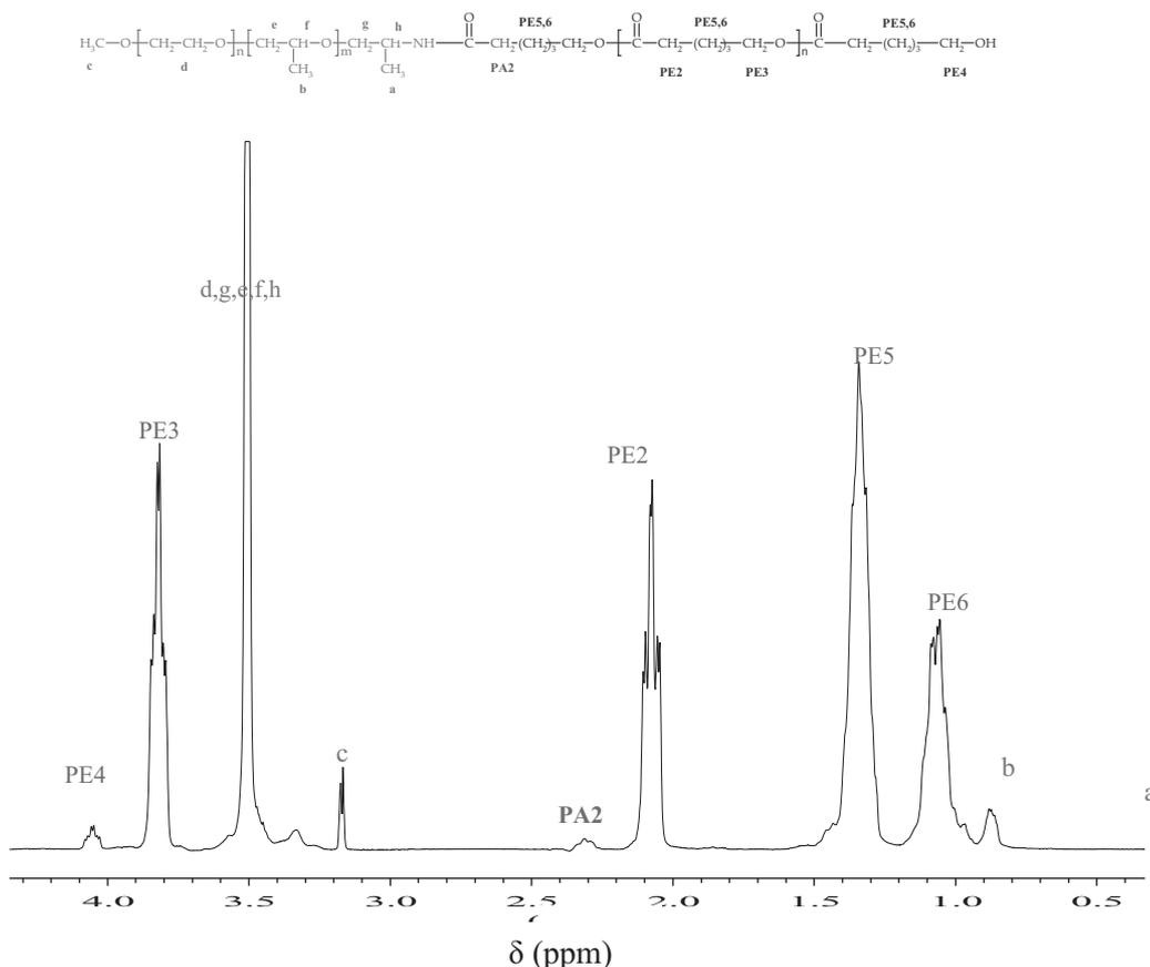
**Figure 2.** <sup>1</sup>H NMR spectrum of a crude polyester as obtained by aminolytic polymerization of CLo initiated by Jeffamine M1000 in the presence of 0.25 mol-% of H<sub>3</sub>PO<sub>2</sub> at 250 °C for 7 h (entry 1, Table 3, solvent: TFA-*d*; 500.13 MHz).
