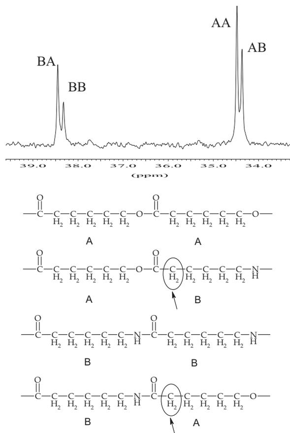
**Figure 4.** Expansion of the 30–40 ppm chemical shift range of a representative  $^{13}\text{C}$  NMR spectrum displaying the  $^{13}\text{C}$  resonances of the  $\text{CH}_2$  groups in  $\alpha$ -position to the carbonyl groups of the copolymer (in a 70:17:13  $\text{CDCl}_3/(\text{CF}_3\text{CO})_2\text{O}/\text{CF}_3\text{COOD}$  mixture) obtained by copolymerization of CLa and CLo initiated by Jeffamine M1000.
