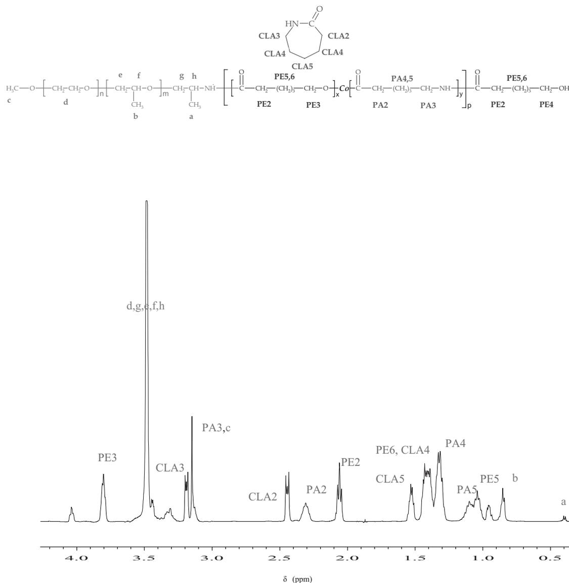
**Figure 3.**  $^1\text{H}$  NMR spectrum of the crude product obtained by copolymerization at  $250^\circ\text{C}$  for 7 h of CLA and CLO, initiated by Jeffamine M1000 in the presence of 0.25 mol-% of  $\text{H}_3\text{PO}_2$  (entry 1, Table 4, solvent: TFA-*d*; 500.13 MHz).
