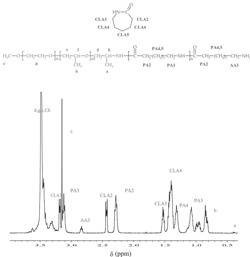
Figure 1. <sup>1</sup>H NMR spectrum of crude polyamide as obtained by aminolytic polymerization of CLA initiated by Jeffamine M1000 in the presence of 0.25 mol-% of H<sub>3</sub>PO<sub>2</sub> at 250 °C for 7 h (entry 4, Table 2, solvent: TFA-*d*; 500.13 MHz).
