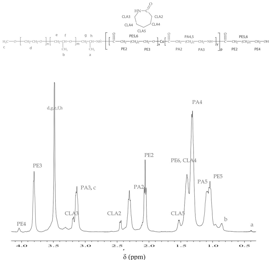
**Figure 5.**  $^1\text{H}$  NMR spectrum of crude product as obtained by simultaneous copolymerization for 24 h of CLA and CLO initiated by Jeffamine M1000 in the presence of 0.50 mol-% of  $\text{H}_3\text{PO}_2$  at  $250^\circ\text{C}$  (entry 2, Table 7, solvent: TFA-*d*; 500.13 MHz).
