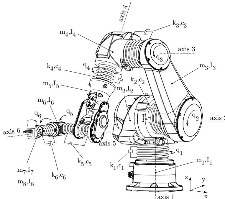
Figure 3: Robot model
