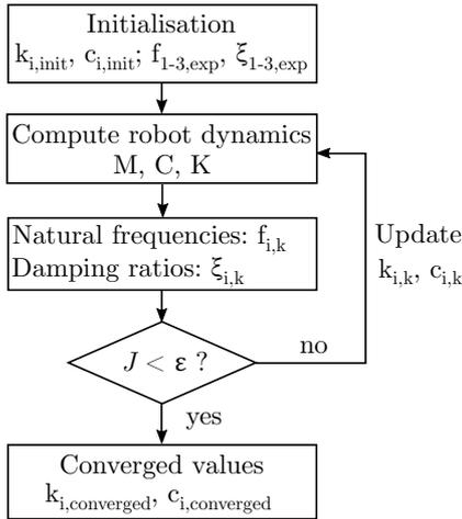
Figure 4: Iterative search of  $k_i$  and  $c_i$
