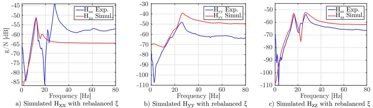
Figure 6: Comparison of FRFs using the rebalanced damping ratios
