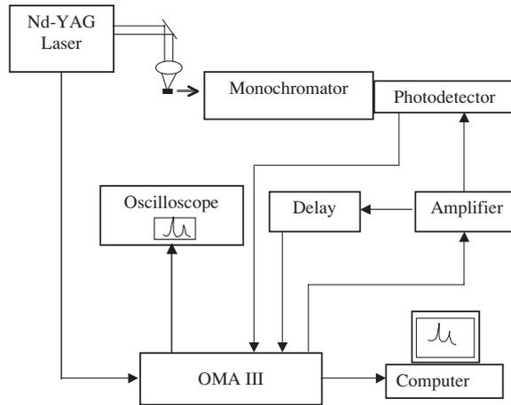
**Figure 2.** Experimental set-up used for branching fraction determination. For a description, see the text.
