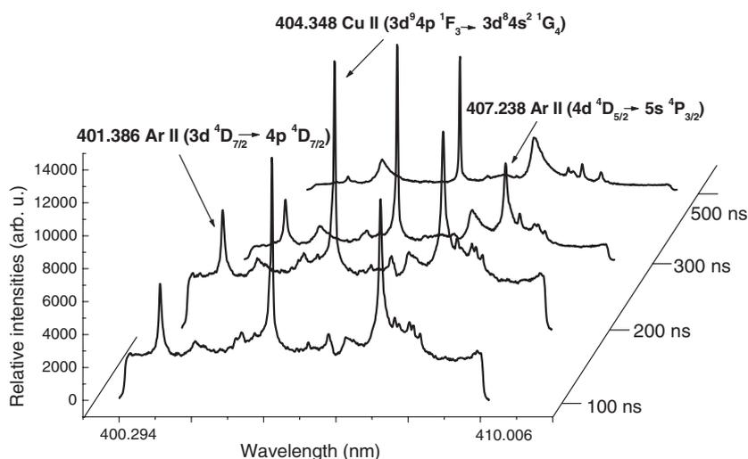
**Figure 3.** Time evolution of the copper spectrum in the region 400 to 410 nm for delay times ranging from 100 ns up to 500 ns.
